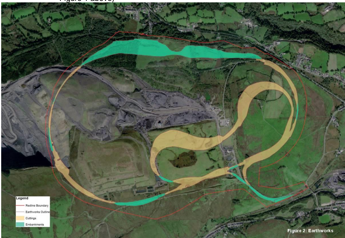
Figure 2: Cuttings and Embankments Aerial (NOTE: The 'red line' shown is NOT the application site boundary for the current application which is correctly identified on Figure 1 above)
